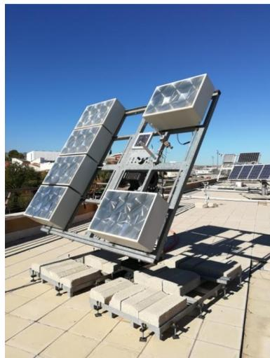
**Figure 7.** The designed high-concentration photovoltaic system (HCPV) tracker.
