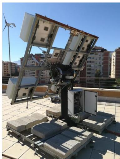
**Figure 8.** The designed high-concentration photovoltaic system (HCPV) tracker.
