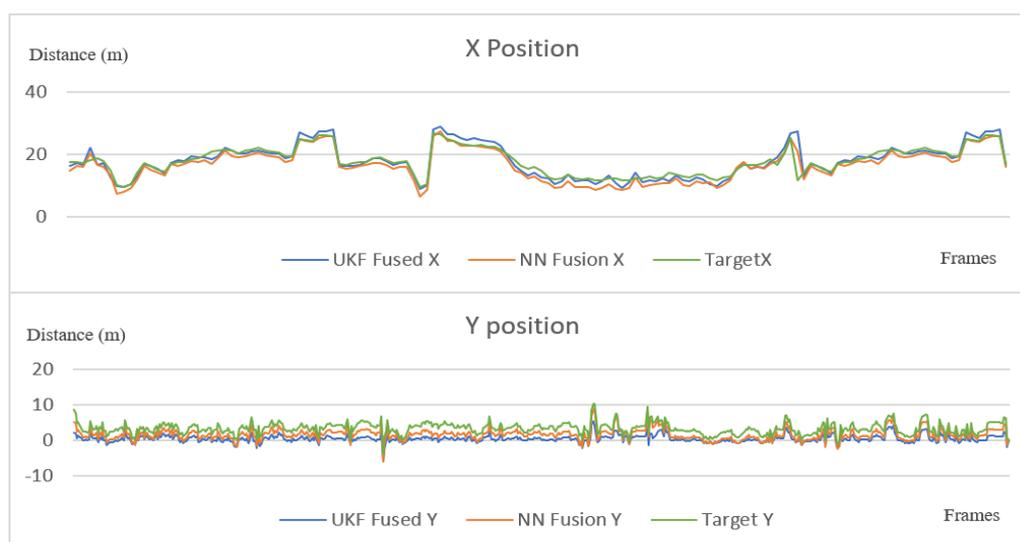
**Figure 22.** Position performance on the  $x$  and  $y$  axes of the proposed sensor fusion methods and the target vehicle.
