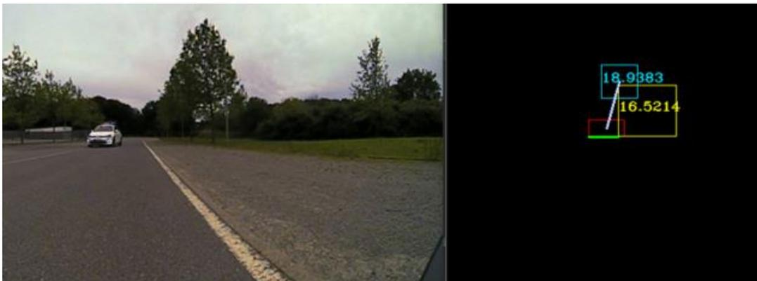
**Figure 8.** Correspondence of the trifocal camera objects and LIDAR and RADAR sensor measurements. On the left-hand side, the color image captured by the camera is shown. On the right-hand image, the data association of objects from different sensors is illustrated.
