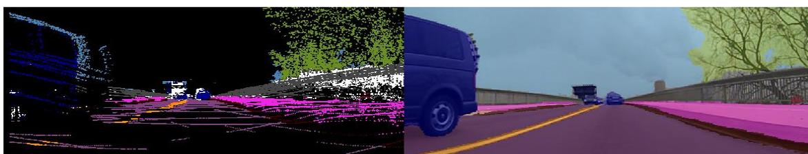
**Figure 10.** Semantic class of each 3D point. On the left-hand side, we observe the assigned semantic class of each projected 3D LIDAR point. In the right image, the semantic class image with 50% transparency is overlapped over the color image.
