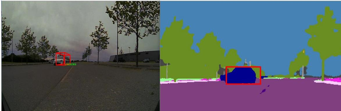
**Figure 18.** Example of mismatch in the validation procedure. On the left-hand side, we observe the projected fused object on the RGB image with the semantic class UNKNOWN. In the right image, the same object is projected onto the semantic class image in a region with the dominant class car. The class mismatch is represented using red color.
