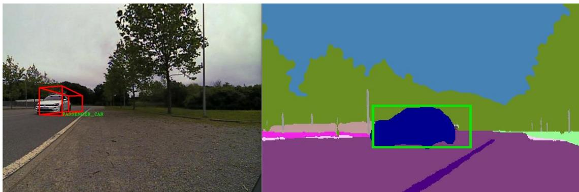
**Figure 19.** Example of successful validation. In the left image, the super-sensor object is projected onto the RGB image. In the right image, the same object is projected onto the semantic segmentation image. The semantic classes’ match is represented using green color.
