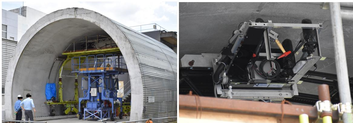
(a) Mock tunnel used in field experiments. Conditions as close as possible of actual inspection sites were realized due to its scale and naturally-occurred defects.
