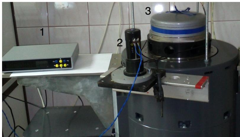
**Figure 2.** Display of the experimental laser dynamic goniometer (LDG) in the mode of an on-axis calibration tool of optical encoders: 1—optical encoder: A-205 processor, 2—DC motor, 3—ring laser.
