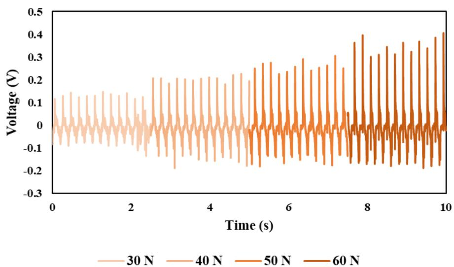
Figure S6. Output voltage under 30 N to 60 N forces and 5 Hz frequency of stretched sample at 50 % strain.
