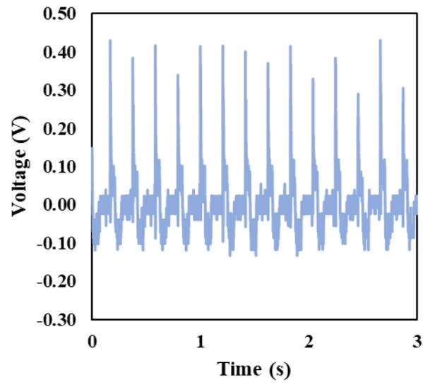
Figure S4. Output voltage under 60 N force and 5 Hz frequency of stretched sample at 100 % strain.
