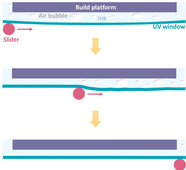
Figure S1. Schematic of the air bubble removal by the sliding process in DLP.
