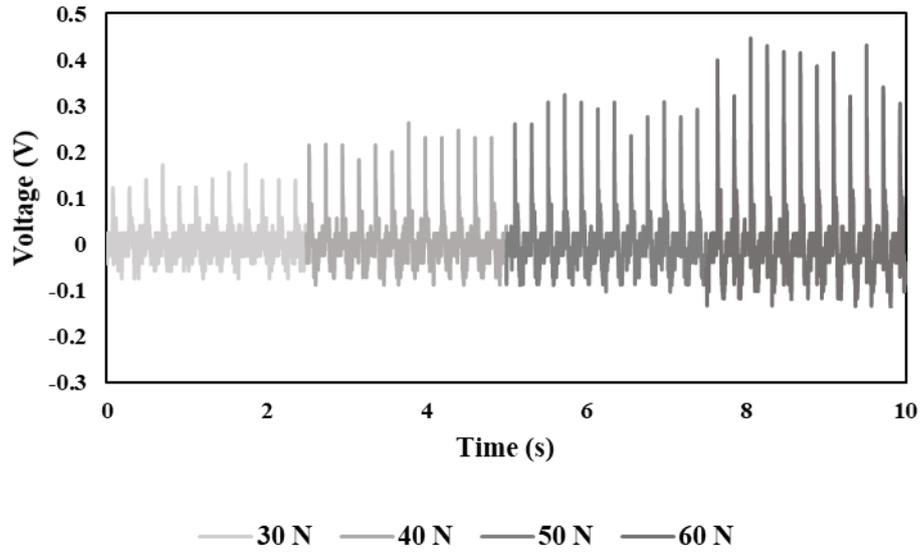
Figure S7. Output voltage under 30 N to 60 N forces and 5 Hz frequency of stretched sample at 100 % strain.
