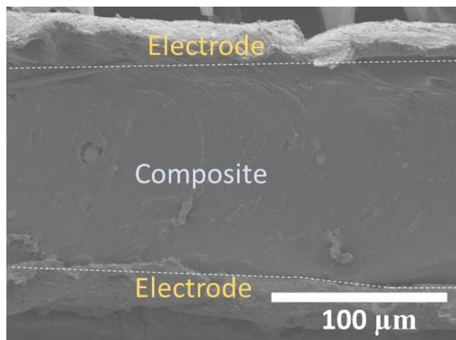
Figure S2. SEM image of the cross-section of the device.
