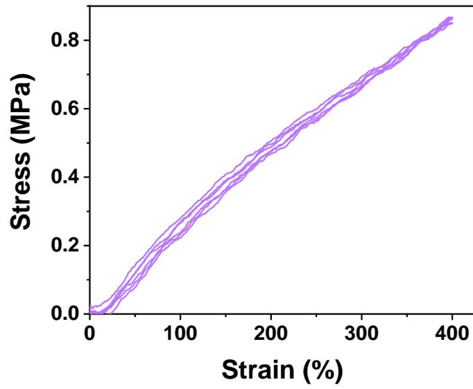
Figure S3. Cyclic tensile testing of the BaTiO<sub>3</sub> NP/EAA/AUD composite (three cycles).
