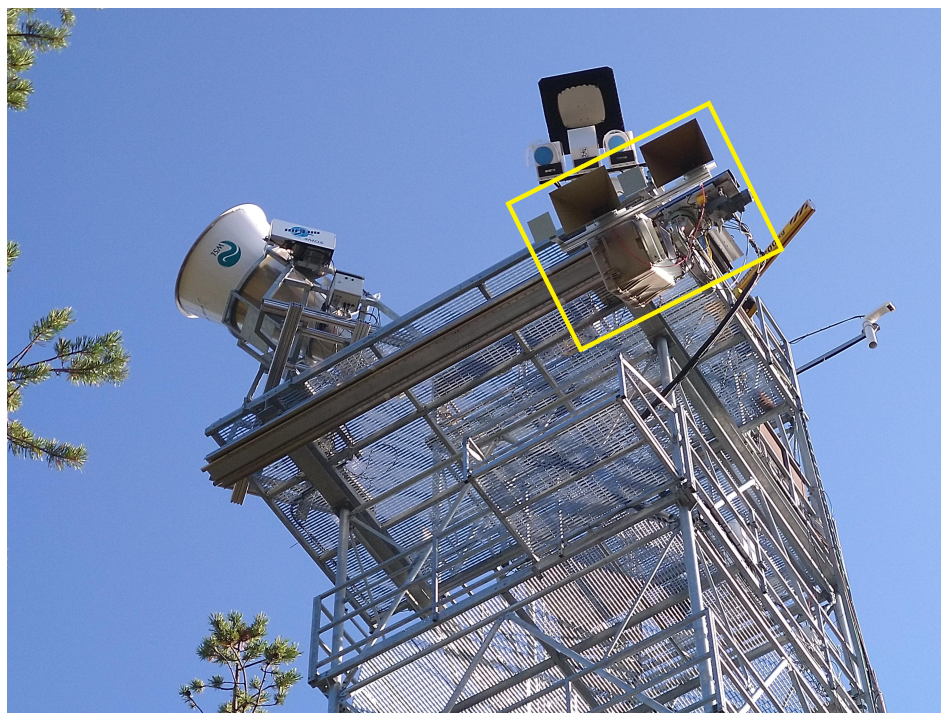
Figure 1. SodSAR mounted on a 21 m tall tower. The radar is mounted on a rail below the platform. Other visible instruments include two passive microwave radiometer systems.
