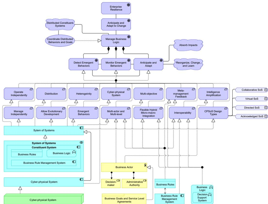
**Figure 5.** Motivation model linking the design goals and requirements to the corresponding architectural building blocks.
