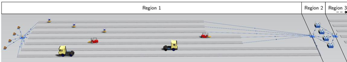
**Figure 8.** A graphical representation of the simulation model. A product flows from region 1 to region 2 after which it undergoes processing. After a product is processed, a transporter moves the cargo from region 2 to region 3. For representation purposes, region 3 is left out of this illustration, but this region is comparable to region 1 (see [20] for more graphical representations).
