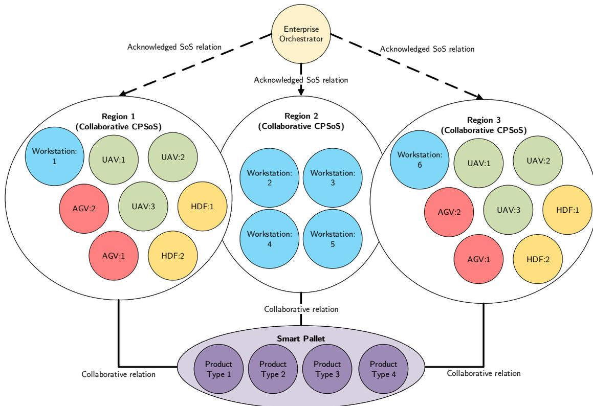
**Figure 7.** Conceptual framework of the case study's constituent systems and CPSoS design relations. Each colored part depicts a constituent system. The smart pallet constituent system contains one of the products, which is considered as a nested constituent system.
