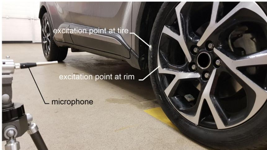
**Figure 6.** Measurement set-up for vibration analysis -points of excitations of vibrations.
