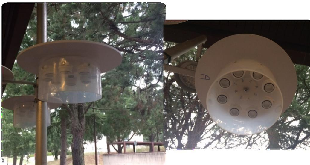
**Fig. S.6.** A pole sustaining up to 3 customized shelters (*on the left*) where each could host up to 8 PASs
