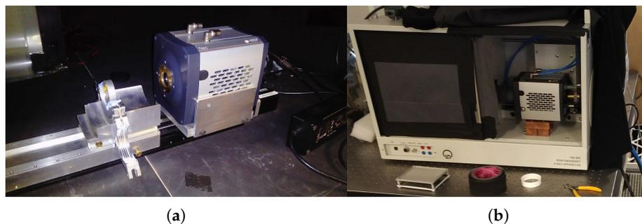
**Figure 1.** (a) Photograph of the source holder and the Neo sCMOS camera in the dark-box. (b) The Neo sCMOS in the LD Didactic X-ray apparatus (554 800)—The blue lines are for the water cooling circuit, which is not necessary for operation in the dark box.
