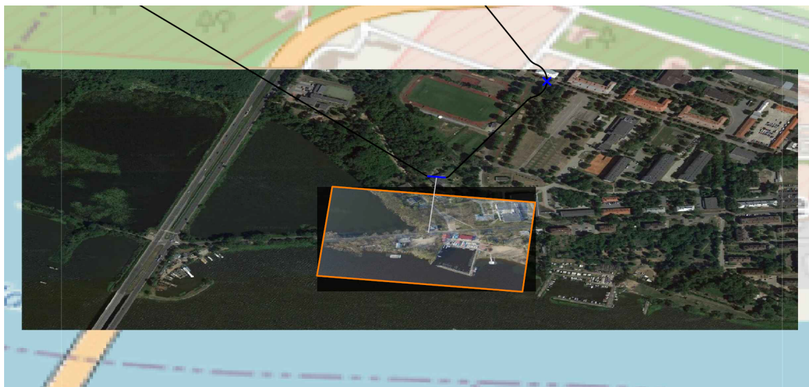
Figure 16. An example of photo data fusion from EO device gathered in different time. UAV trajectory segments are marked. The smaller photo was taken by UAV for recognition of objects located in this smaller area.
