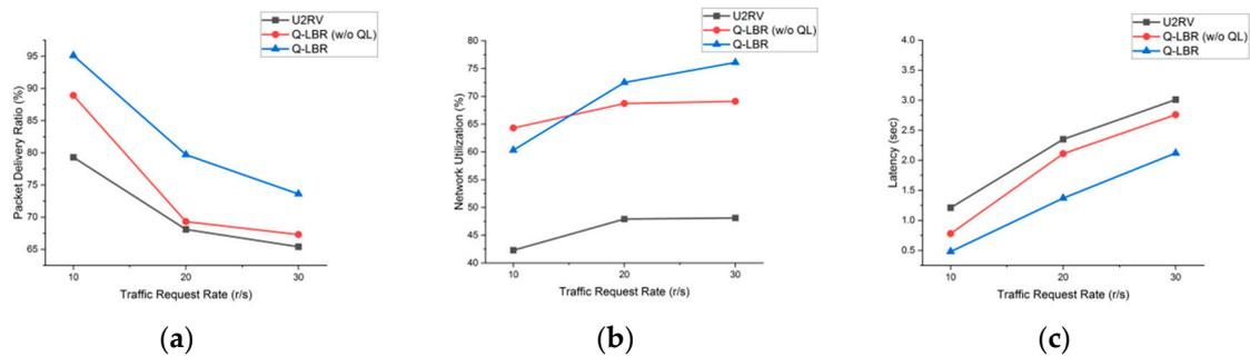
**Figure 11.** Performance comparison for traffic request rate: (a) total PDR, (b) total network utilization and (c) total latency.
