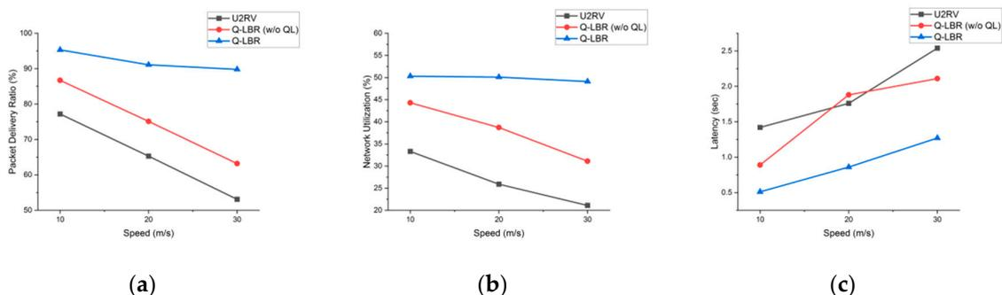
Figure 10. Performance comparison for ground node speed: (a) total PDR, (b) total network utilization, and (c) total latency.
