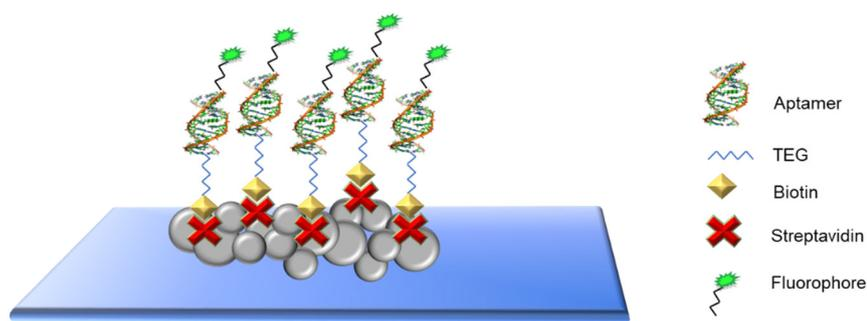
**Figure S4.** Sketch of the biotin-streptavidin pairing strategy. The aptamers are functionalized with biotin-TEG 5' and the ns-ZrO<sub>2</sub> is coated with streptavidin. The 15-atom tetraethylene glycol (TEG) spacer is added for minimizing steric hindrance when conjugating the biotin with other molecules.
