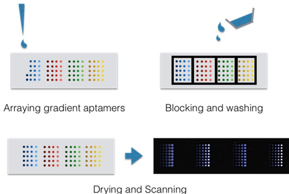
**Figure S1.** Sketch of PSIM protocol applied to one fluorescent aptamer spotted on ns-ZrO<sub>2</sub> at different concentrations. Upper left: spotting; upper right: incubation in a controlled atmosphere (65% humidity), immersion in a blocking solution and rinsing; bottom left: drying and bottom right: scanned image.
