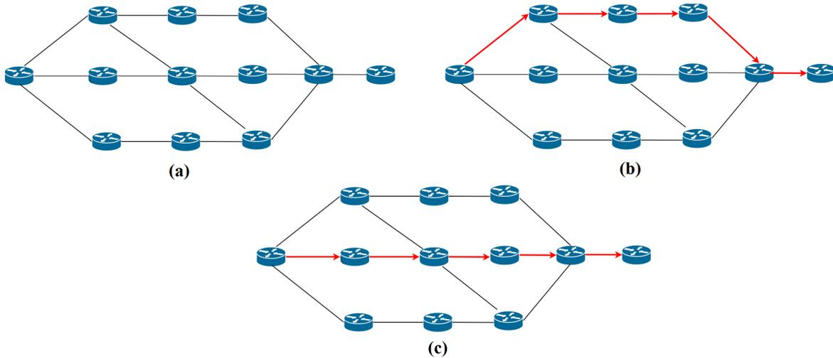
**Figure 5.** (a) Original Topology. (b) Shortest Path. (c) Shortest path determined using Algorithm 2 in our example scenario.
