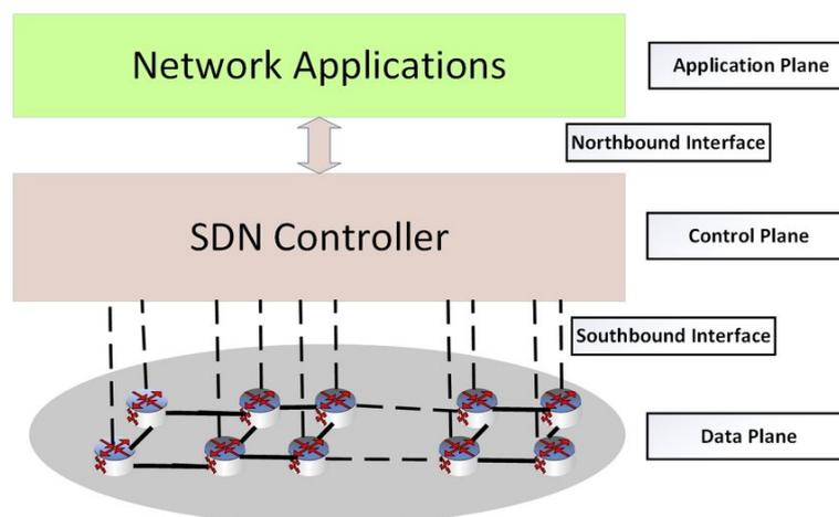
**Figure 1.** Software-defined network (SDN) architecture.
