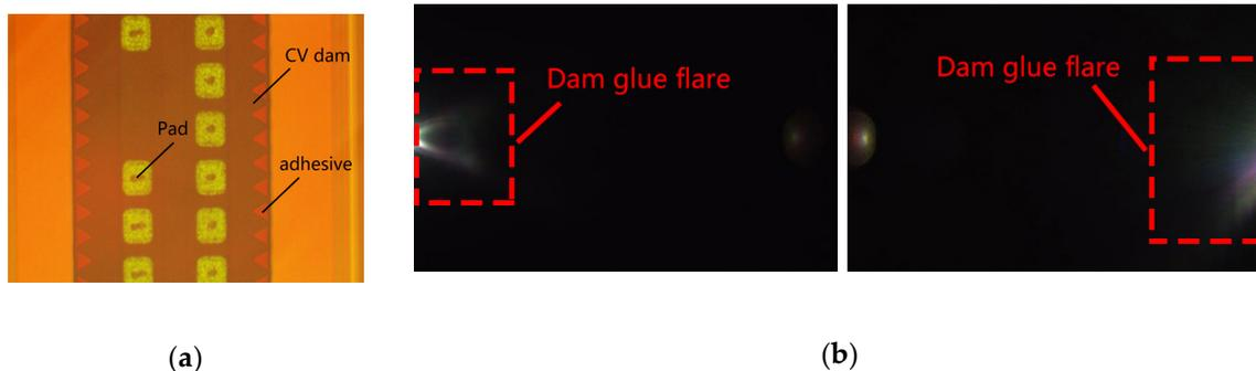
**Figure 9.** (a) Adhesive overflowed the CV dam; (b) flare image issue caused by dam glue reflection.
