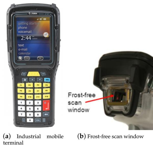
**Figure 1.** A typical industrial mobile terminal used for low-temperature operation: Zebra Omnii XT15f.
