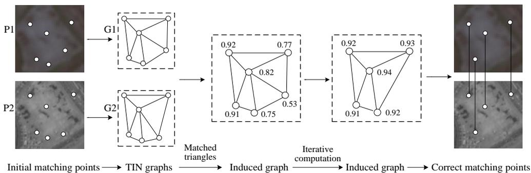
Figure 2. The workflow of triangular irregular network (TIN) graph.
