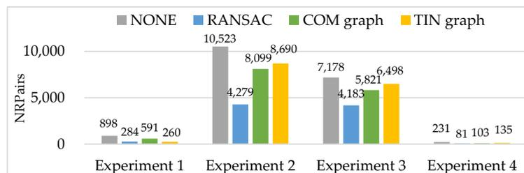
**Figure 9.** Experimental results of the number of remaining matching point pairs (NRPairs).
