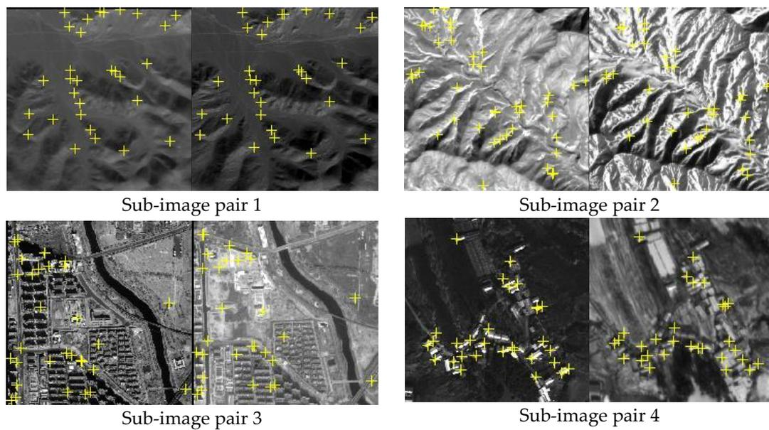
**Figure 5.** Manually measured tie points (yellow crosses) in four sub-image pairs.
