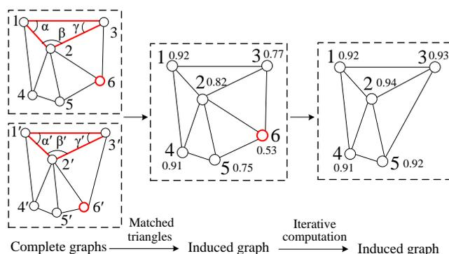
Figure 3. The main workflow of building and iterating the induced graph.
