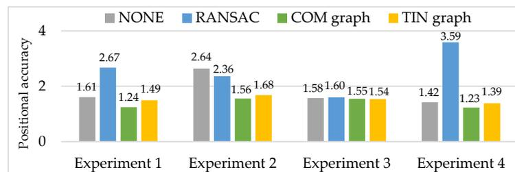
Figure 11. Experimental results of positional accuracy (RMSE, pixel).
