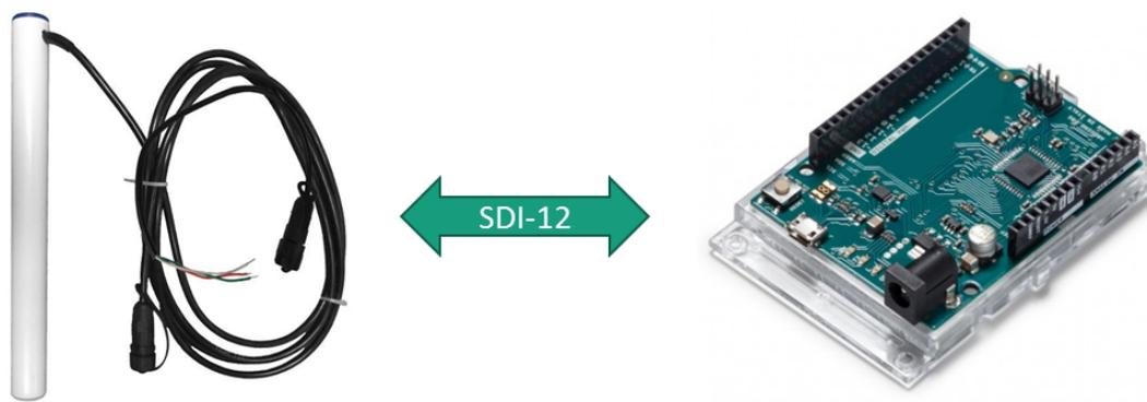
Figure 10. Prototype for soil moisture sensor.
