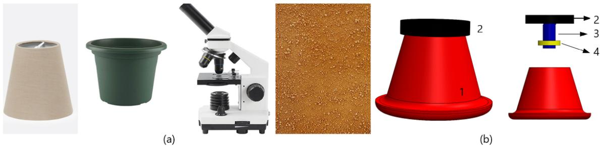
**Figure 7.** (a) Inspiration board. (b) Initial casing concept diagram: (1) Cabinet; (2) Sensing box casing; (3) Camera; (4) LEDs.
