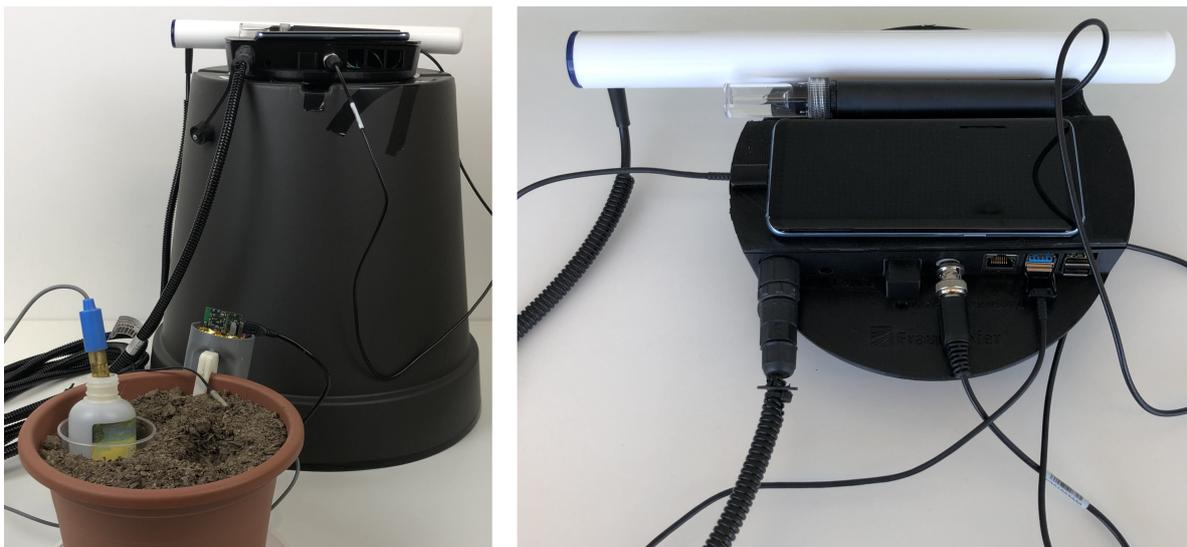
**Figure 16.** IoT sensing platform fully assembled prototype.
