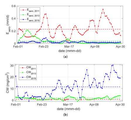
**Figure 7.** (a) Daily evaporation rate ( $E_{aero}$ ) and (b) daily condensed water (CW) before (2011) and after the intervention of maintenance (2013–2019). Average values are represented as dashed lines.
