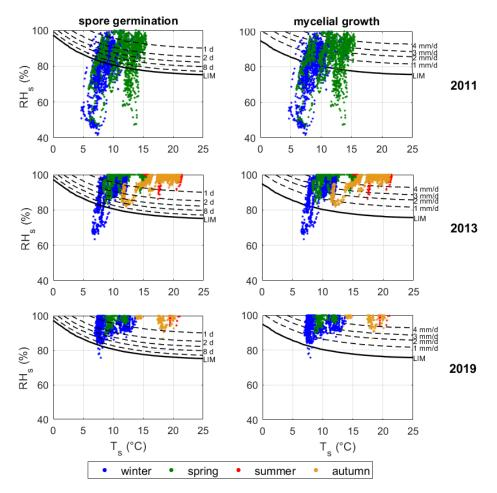
**Figure 9.** Relative humidity ( $RH_s$ ) *vs* temperature ( $T_s$ ) close to wall surfaces plotted on Sedlbauer curves (isopleths) for mould risk assessment on Substrate category I. Left panels: mycelial growth curves in mm/d; right panels: spore germination curves in days.
