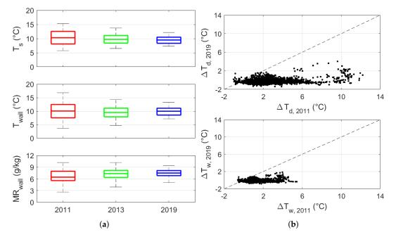
**Figure 6.** (a) Boxplots of wall surface temperature ( $T_s$ ), air temperature (T), and mixing ratio (MR), and (b) scatterplots of temperature difference between  $T_s$  and  $T_d$ , i.e.,  $\Delta T_d$ , and temperature difference between  $T_s$  and  $T_w$ , i.e.,  $\Delta T_w$ .
