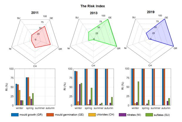
**Figure 10.** Comparison among Risk Index (RI) values calculated for individual risks before (2011) and after (2013-2019) the maintenance intervention. Upper panels: radar plot with RI (%) calculated on a yearly basis. Lower panels: histogram plots of RI (%) calculated on a seasonal basis.
