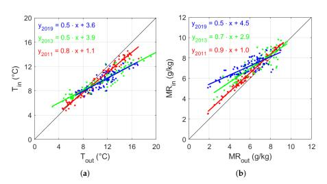
**Figure 4.** Scatter plot of daily mean indoor values *versus* outdoor values collected from 1st February until 30th April in 2011, 2013, and 2019: (**a**) air temperature (T) and (**b**) mixing ratio (MR). The linear regression equations for each dataset are reported together with the bisectrix (i.e.,  $T_{in} = T_{out}$  and  $MR_{in} = MR_{out}$ , in black).
