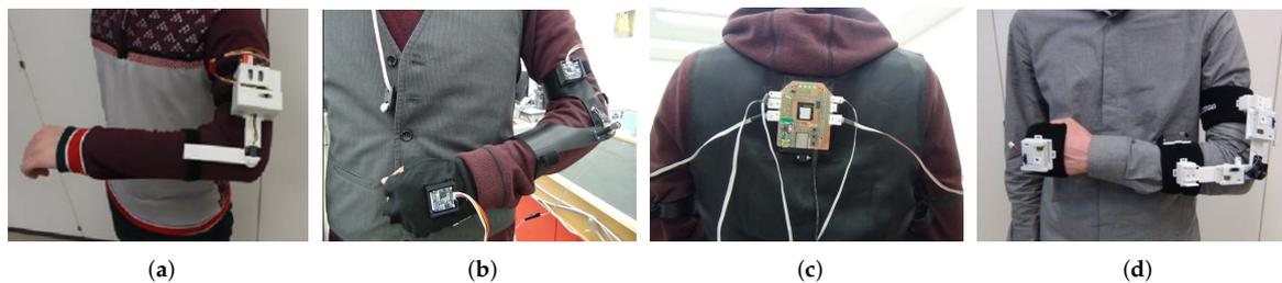
**Figure 2.** Evolution of the arm motion-tracking system designs: (a) the 4-DOF system (Phase 1) [22]; (b,c) the 7-DOF double-arm system used in [30] (Phase 2); (d) the final 7-DOF system (Phase 3) used in [31].
