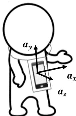
**Figure 1.** Smartphone sensor worn around the neck. The three axes of the built-in accelerometer are indicated by  $(a_x, a_y, a_z)$ .
