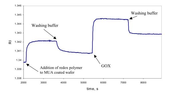
**Figure 3**. Changes in refractive index with time as measured by SPR during the assembly of a nanocomposite thin film consisting of MUA and one RP/GOX bilayers. The concentrations of RP and GOX were 10 mg/mL in PBS, flow rate 80  $\mu$ L/min.
