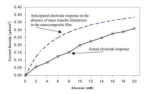
**Figure 5.** Concentration dependence of the electrode current density for a nanocomposite thin film comprised of two RP/GOX bilayers. The solid line shows the actual response of a nanocomposite thin film while the dash line shows the anticipated response in the absence of mass transfer limitations in the film. Currents were acquired using cyclic voltammetry (0 to 500 mV, 20 mV/s), with the current at 500 mV used in the current density calculation.
