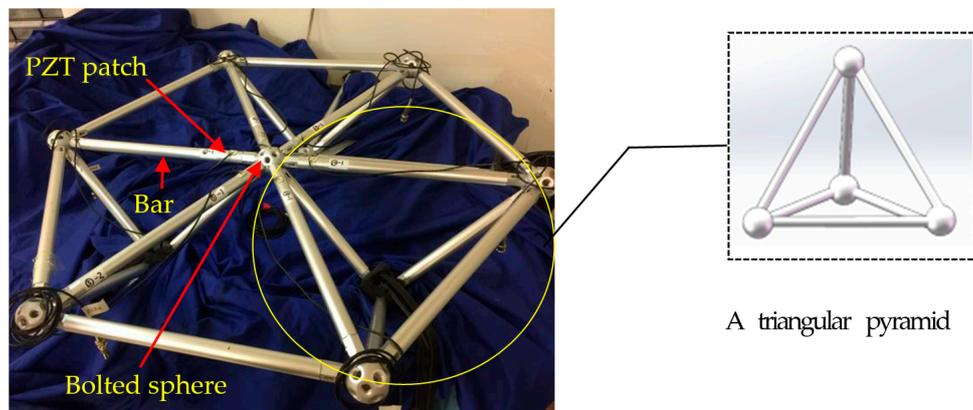
Figure 3. Photo of triangle-on-triangle offset grid specimen.
