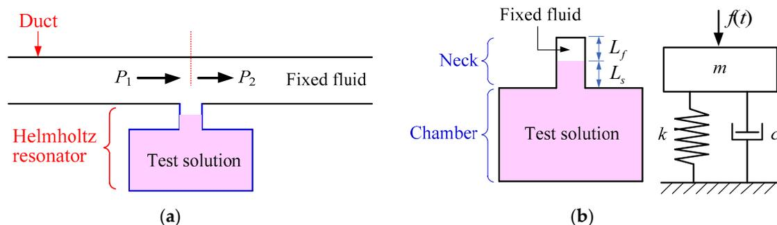
**Figure 1.** (a) The Helmholtz resonator linked with a duct; (b) Structure of Helmholtz resonator and its equivalent mass-spring model.
