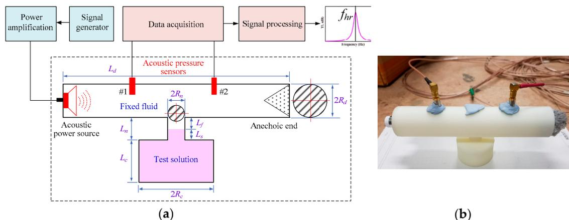
**Figure 2.** (a) Schematic illustration of analyte concentration measurement in the test solution; (b) Device architecture of the duct linked with a Helmholtz resonator.
