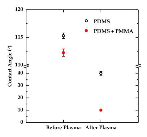
**Figure S2.** Contact angle for PDMS films and PDMS films coated with PMMA, before and after being subjected to an oxygen plasma treatment. Note that the values represented correspond to average values ± standard deviation of a minimum of 6 measurements. For PDMS films coated with PMMA, the contact angle after the oxygen plasma treatment is represented as being 10°, however, the real value is smaller but it cannot be precisely estimated due to technique limitations.
