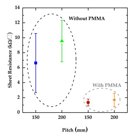
**Figure S1.** Sheet resistance of carbon coating on micro-structured s-PDMS films. Note that the values represented correspond to average values ± standard deviation of a minimum of 3 films.
