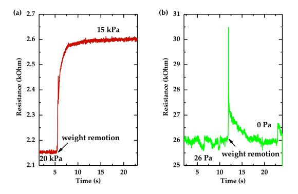
**Figure S3.** Resistance change when removing weights from the top of sensors. (a) Resistance change from 20 kPa to 15 kPa of a sensor with a PMMA layer and a semi-spheres theoretical pitch of 150  $\mu$ m. (b) Resistance change from 26 Pa to 0 Pa of a sensor without a PMMA layer and with a semi-spheres theoretical pitch of 200  $\mu$ m.
