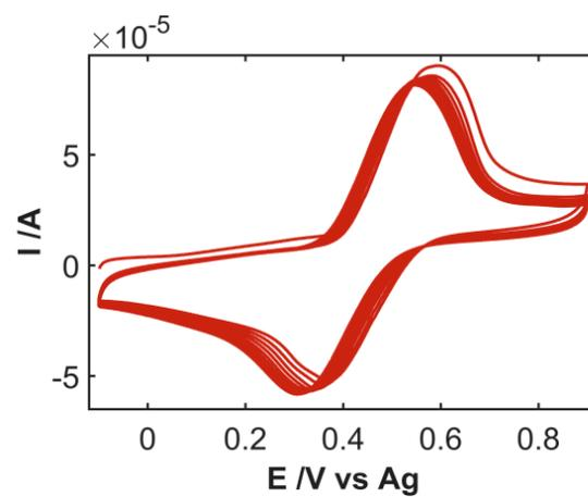
**Figure S3.** CV response of 10<sup>-3</sup> M CFA, 0.1 M acetic acid solution at SWCNT<sub>ox</sub> electrode between -0.10 and +0.90 V at 0.02 Vs<sup>-1</sup>.
