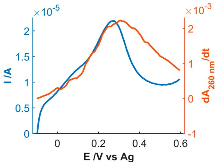
**Figure S6.** Comparison of LSV and derivative voltabsorptogram at 260 nm during the oxidation of  $3 \cdot 10^{-4}$  M NADH, 0.1 M PBS.
