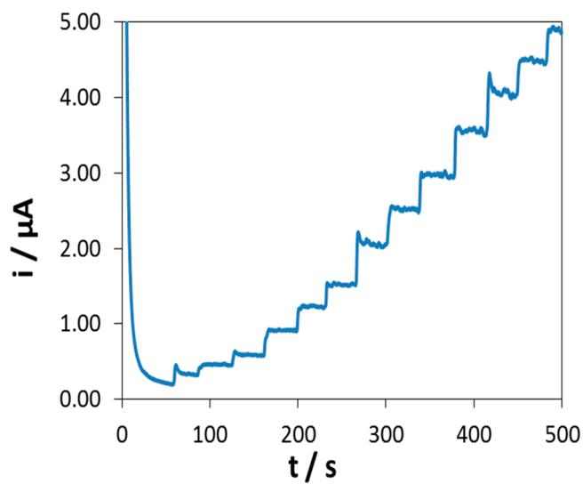
**Figure S5.** Amperometric response recorded with SWCNT<sub>CFA</sub> at +0.30 V in stirred 0.1 M PBS, by subsequent additions of defined aliquots of a NADH solution.
