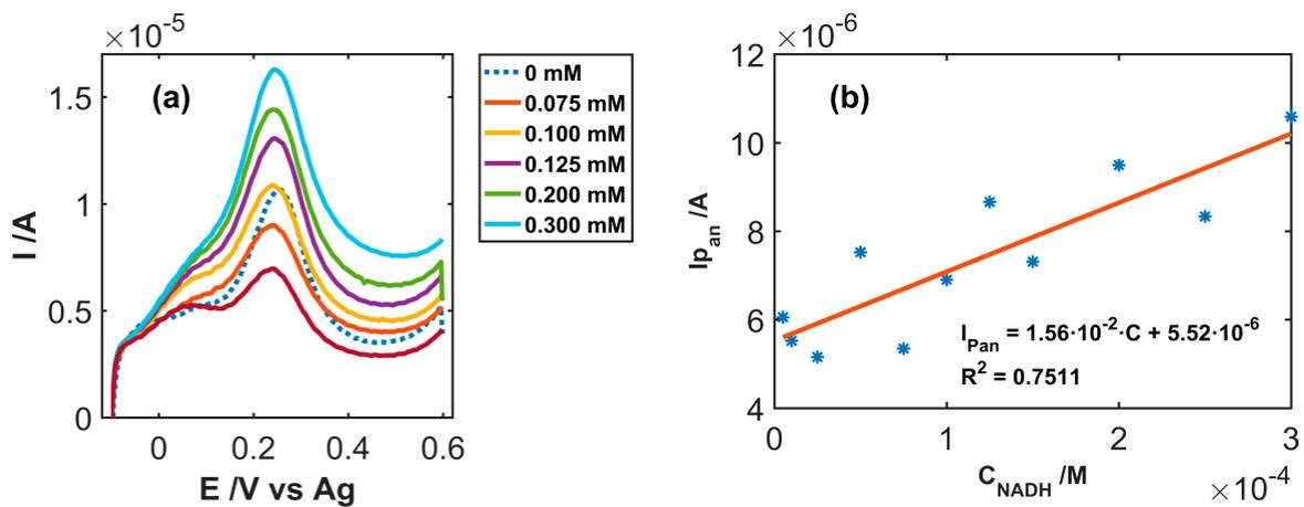
**Figure S7.** (a) LSV registered during the oxidation of  $2 \cdot 10^{-4}$  M NADH in 0.1 M PBS. (b) Calibration curve of the current peak values *vs* the NADH concentration.
