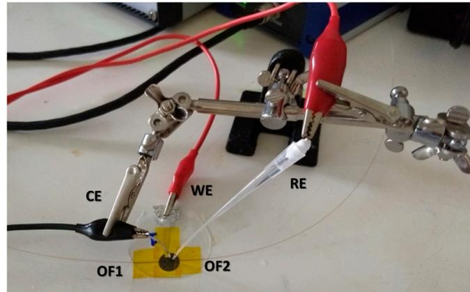
**Figure S2.** Photograph of the UV/Vis absorption spectroelectrochemical set-up in parallel configuration. WE: SWCNT working electrode, CE: Pt counter electrode, RE: Ag/AgCl/KCl 3M reference electrode, OF1: naked optical fibre that guides the light beam from the source cell to the solution, OF2: naked optical fiber that guides the light beam from the solution to the spectrometer.
