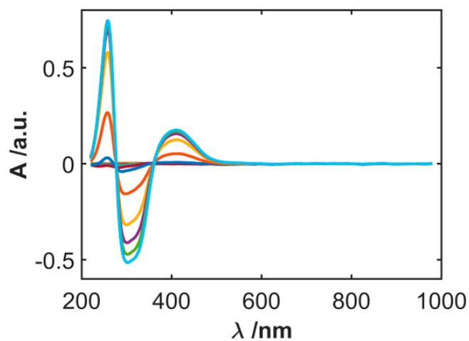
**Figure S4.** UV-Vis absorption spectra recorded during the first scan toward positive potential values at SWCNT<sub>ox</sub> electrode in  $10^{-3}$  M CFA, 0.1 M acetic acid solution, between -0.10 and +0.90 V at  $0.02 \text{ V s}^{-1}$ .
