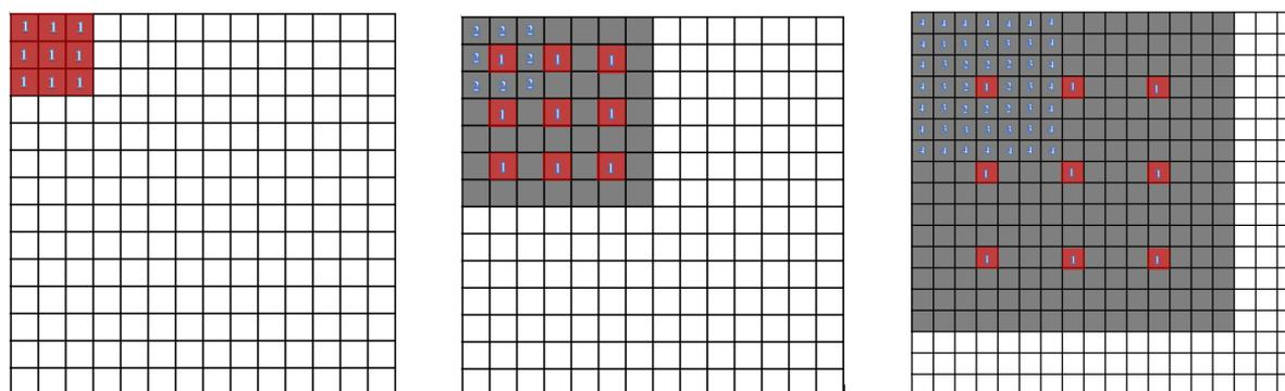
(a) Conventional convolution  $d = 1$ (b) Dilated convolution with  $d = 2$ (c) Dilated convolution with  $d = 4$
