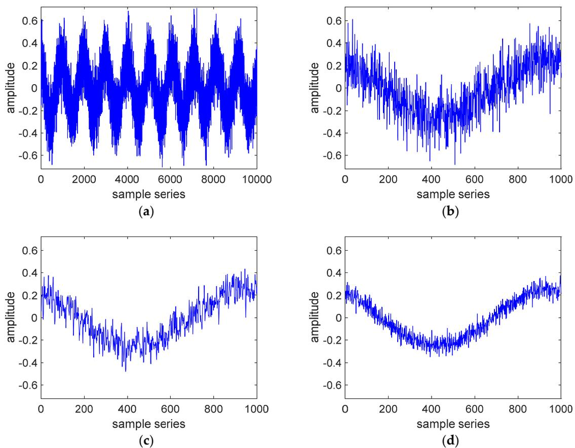
**Figure 2.** Comparison of the signals before and after limited recursive average filtering and coherent accumulation: (a) simulated sinusoidal signal with noise; (b) zoomed-in view of one cycle of (a); (c) one cycle of the filtered signal by limited recursive average filtering (LRAF); (d) one cycle of the filtered signal by coherent accumulation (CA).
