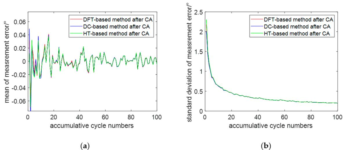
**Figure 5.** Effects of the different accumulation cycles on each method: (a) mean of measurement error; (b) standard deviation of measurement error.
