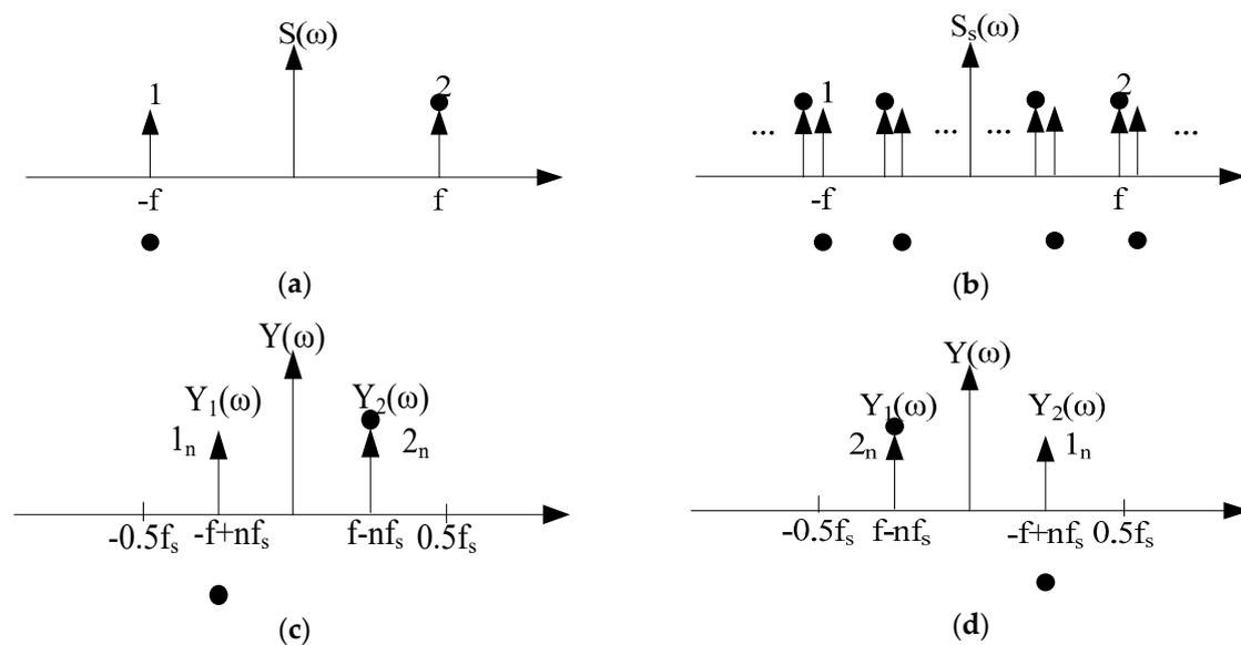
**Figure 1.** Signal spectrum schematic: (a) Original signal spectrum; (b) signal spectrum after sampling; (c) signal spectrum after low-pass filtering (case 1); (d) signal spectrum after low-pass filtering (case 2).
