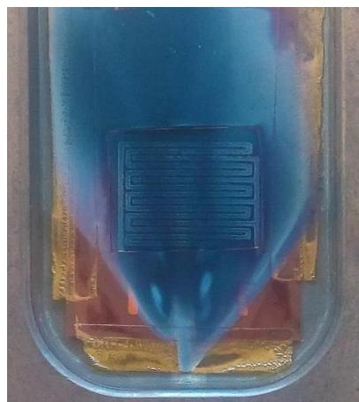
**Figure 1.** View of the steel hot wall reactor, opened after the aerosol-assisted chemical vapor deposition (AA-CVD) process. Kapton mask (brown), Ag stenciled tracks, and grown  $\text{WO}_3$  (blue) can be observed.
