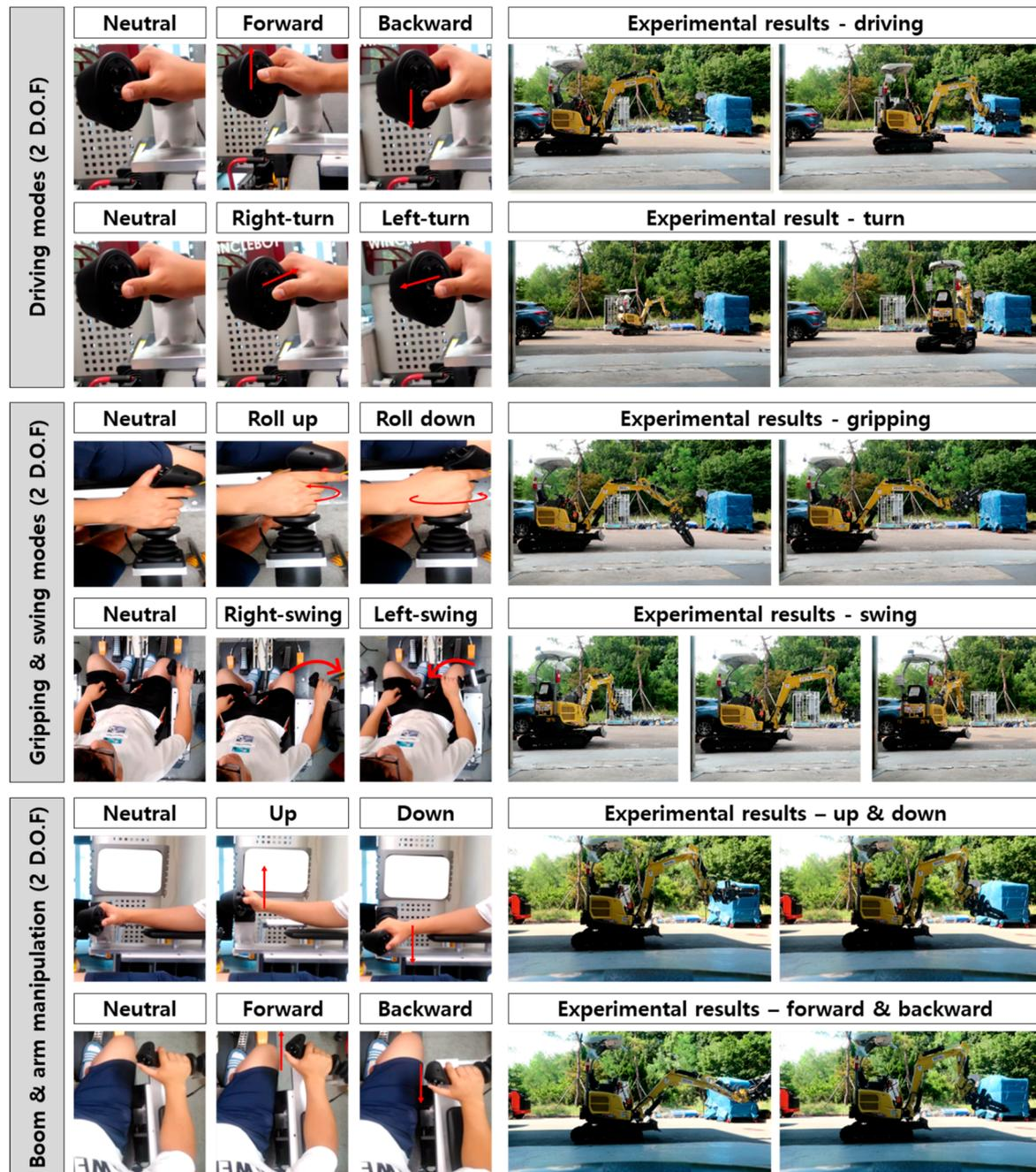
Figure 8. Excavator operation test based on 6 D.O.Fs.
