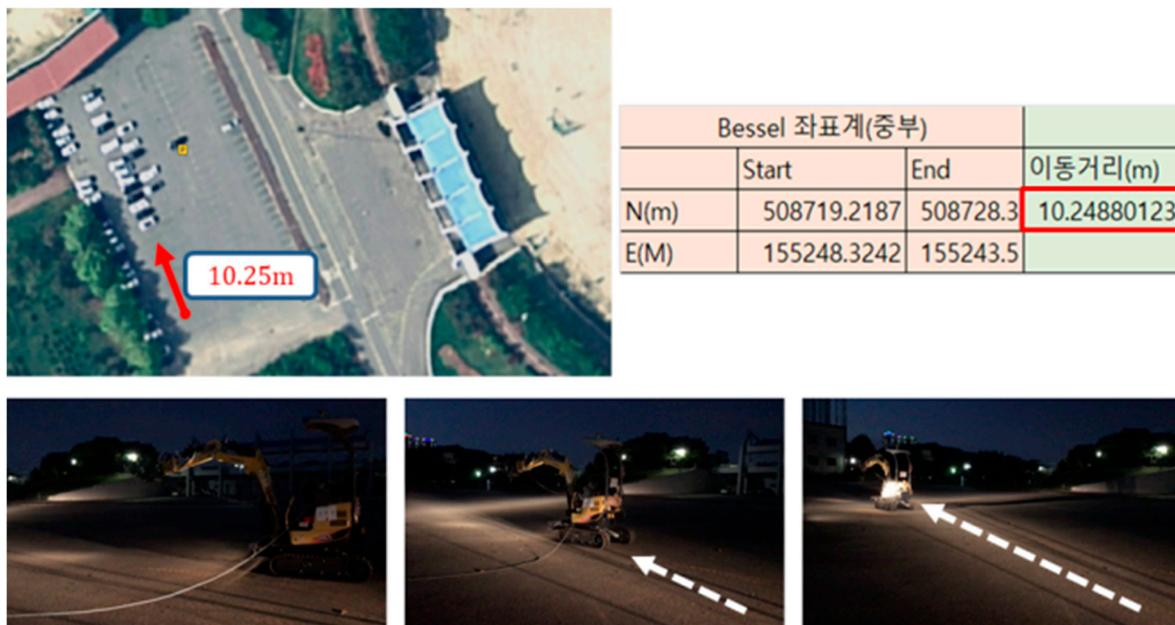
Figure 12. Maximum acceptable distance between the operator and the unmanned vehicle.
