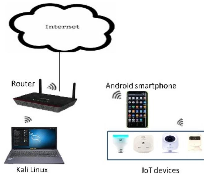
Figure 3. IoT smart-home testbed network architecture.
