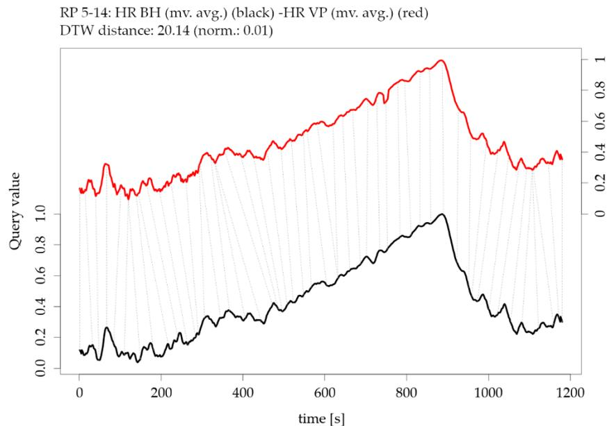
**Figure 15.** Illustration of the Dynamic Time Warping (DTW) distance between two parameters of participant RP 5-14: moving averaged version of heart rate HR from BioHarness BH versus moving averaged version of heart rate HR from VarioPort VP (note the offset of the two y-axes).
