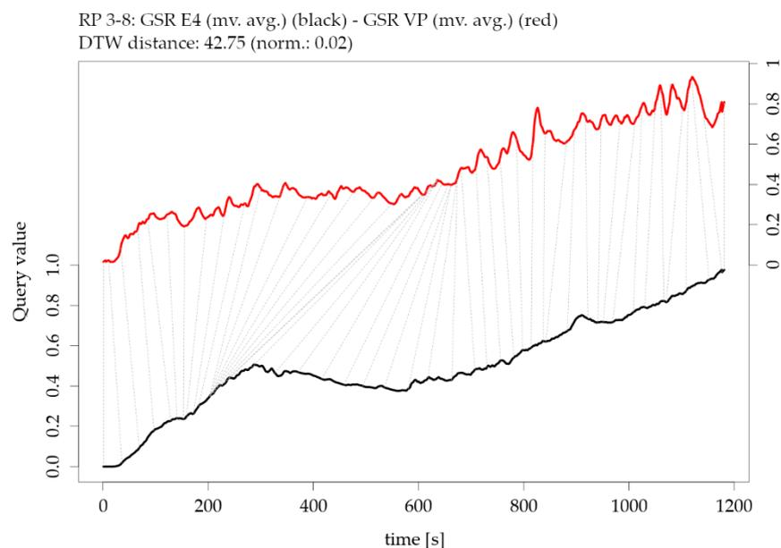
**Figure 16.** Illustration of the Dynamic Time Warping (DTW) distance between two parameters of participant RP 3-8: moving averaged version of galvanic skin response GSR from E4 versus moving averaged version of galvanic skin response GSR from VarioPort VP (note the offset of the two y-axes).
