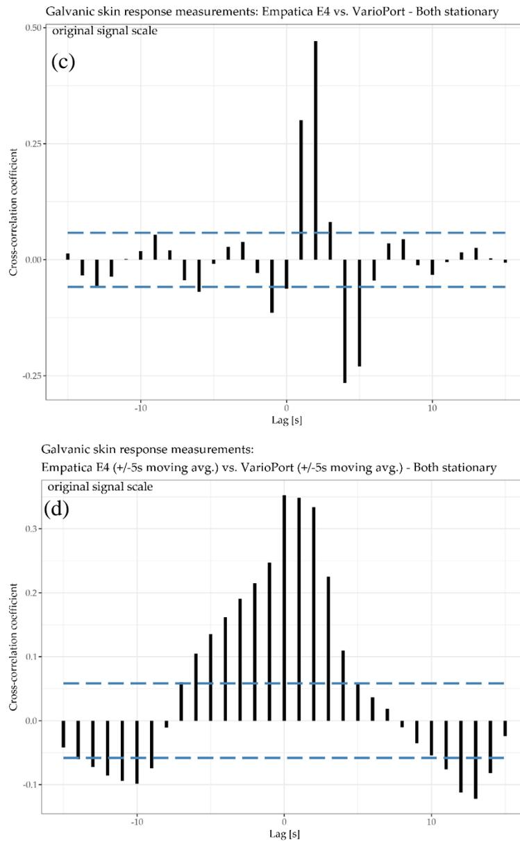
**Figure 5.** Participant RP 3–8: time plots (a), scatter plot (b), cross-correlation plot (c), and cross-correlation plot of moving averages (d) of galvanic skin response GSR measured by Empatica E4 and VarioPort.
