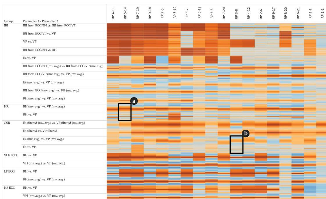
**Figure 7.** Cross-correlation matrix of pairs of parameters and participants; detail (a) complements Figure 4, detail (b) complements Figure 5; colour: orange indicates positive cross-correlation, blue indicates negative cross-correlation; a cell detail shows lags as small horizontal bars: lag -15 at top, and lag +15 at bottom.
