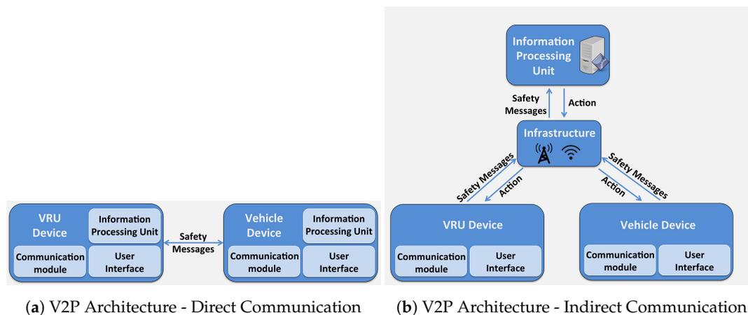
**Figure 2.** Example V2P System Architectures.
