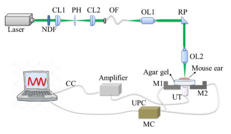
**Figure 1.** The home-made optical-resolution photoacoustic microscopy (PAM) imaging system. NDF: Neutral density filter; PH: pinhole; CL1 and CL2: Convex lens; OF: Optical fiber; OL1 and OL2: Objective lens; RP: Rectangular prism; M1 and M2: Two-dimensional motor; MC: Motor Control; UT: Ultrasonic transducer; UPC: Ultrasonic probe cable; and CC: Coaxial cable.
