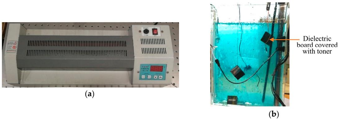
Figure 8. The equipment used to produce the patch antenna. (a) a thermal transfer printer; (b) corrosive liquid.
