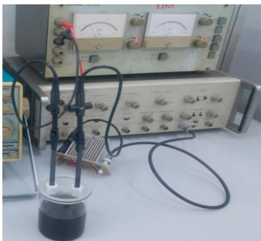
**Figure 1.** Experimental set-up employed for graphite electrochemical exfoliation by pulses of current (0.5 A intensity; 2.5 s pulse duration; 0.8 s pause between two pulses).
