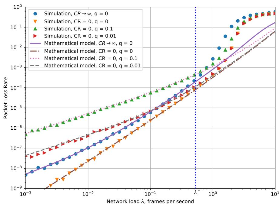
**Figure 6.** Dependency of packet loss ratio (*PLR*) on the cumulative network load.
