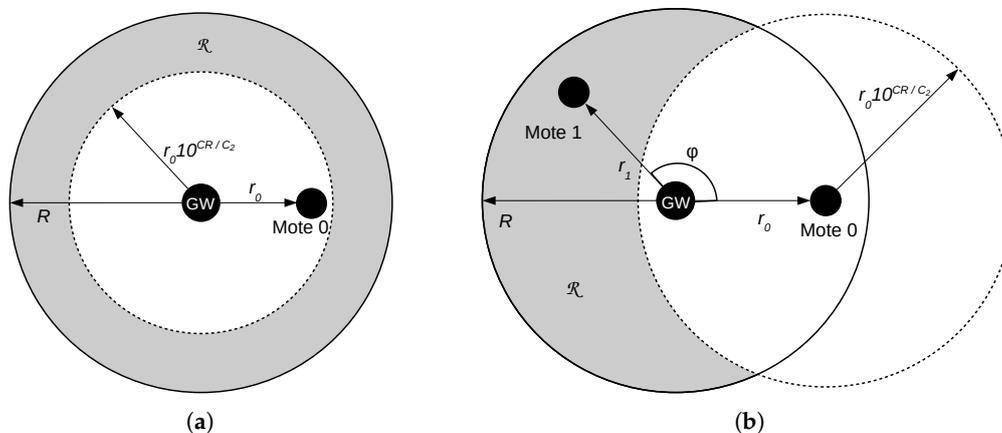
**Figure 4.** Mote locations for various cases: (a) mote 1 location when data frame of Mote 0 is successful in case of collision. (b) Mote 1 location when ACK is successful if it collides with data.
