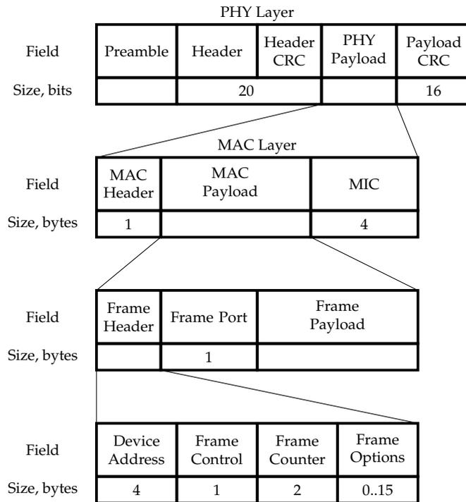
Figure 1. LoRaWAN Frame Format [4].
