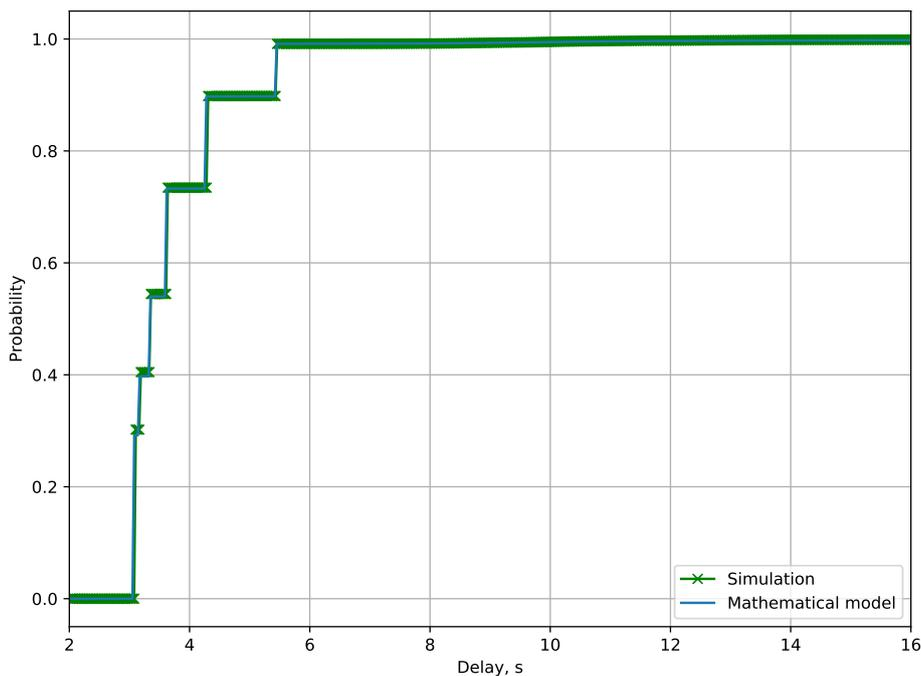
Figure 8. Packet delivery time cumulative distribution function for  $\lambda = 0.4$  frames per second.
