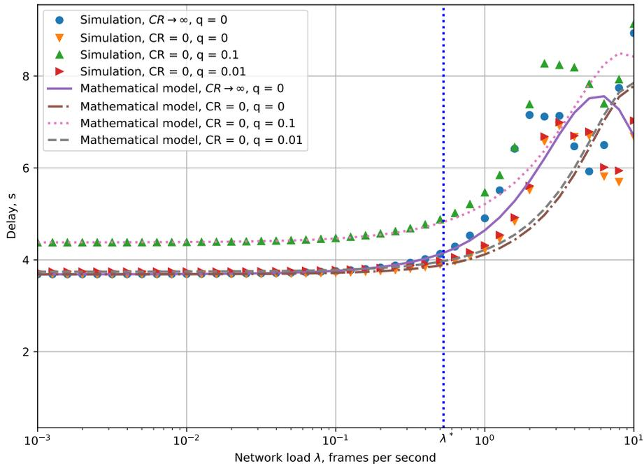
Figure 7. Dependency of the packet delivery time on the network load.
