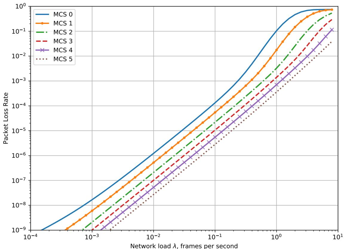
**Figure 9.** Dependency of PLR on the network load for various MCSs,  $CR = 6$  dB.
