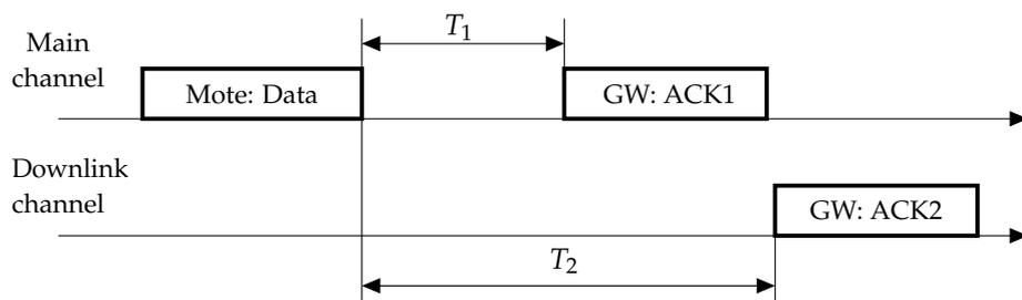
Figure 2. Data transmission and acknowledgment in a LoRaWAN network.
