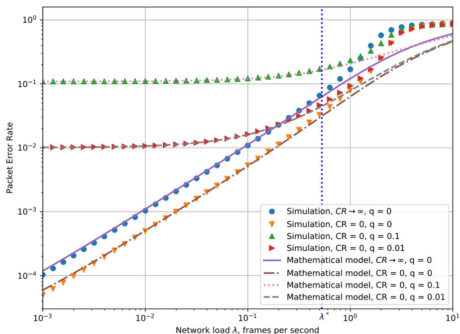
**Figure 5.** Dependency of packet error rate (PER) on the cumulative network load.
