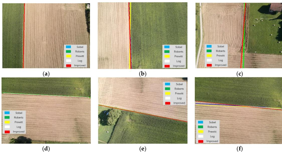
**Figure 23.** Comparison between the improved anti-noise morphology algorithm and existing operators using standard datasets. Red navigation lines were created using the improved anti-noise morphology algorithm: (a) first image sample; (b) second image sample; (c) third picture sample; (d) fourth picture sample; (e) fifth picture sample; (f) sixth picture sample.
