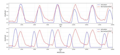
**Figure 5.** The activations on the first ReLU of respiration (RESP) signal. To easily see which signal patterns were activated, the activations and the first batch-normalization layer's outputs were normalized with MinMax Scaler having a range from 0 to 1. The blue line indicates the activations and the red line indicates the output. Activations around (**a**) RESP peak (e.g., inspiration) and (**b**) RESP nadir (e.g., expiration).
