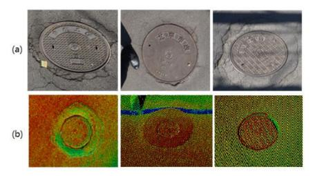
Figure 4. Example manhole-cover images. (a) Ground images. (b) Laser data images.
