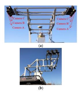
**Figure 2.** Structure of the reconstructed camera system and mounting frame. (a) Bottom view of the modified system. (b) Side view of the modified system.
