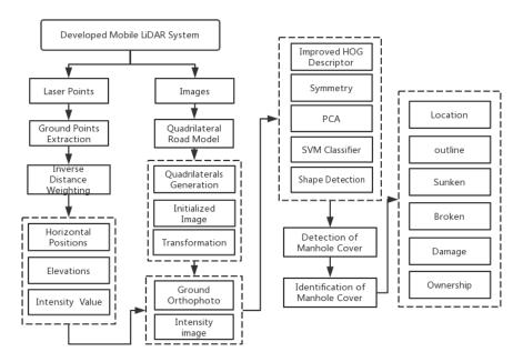
**Figure 5.** Framework for manhole cover detection and identification.
