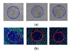
Figure 11. Detection of the manhole cover outline. (a) Ground image examples. (b) Laser data examples.
