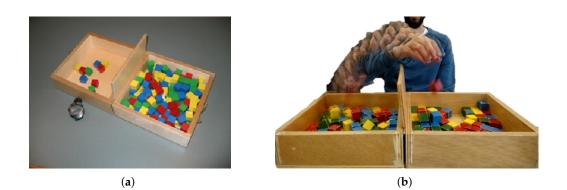
Figure 1. Box and Blocks Test. (a) Components: wooden box, coloured cubes and stopwatch; (b) user during test development.
