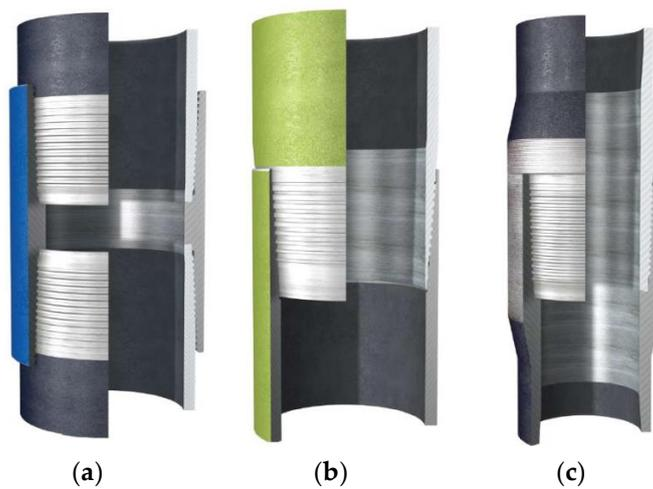
**Figure 1.** (a) Threaded and coupled, (b) integral flush, (c) integral upset connection [35].
