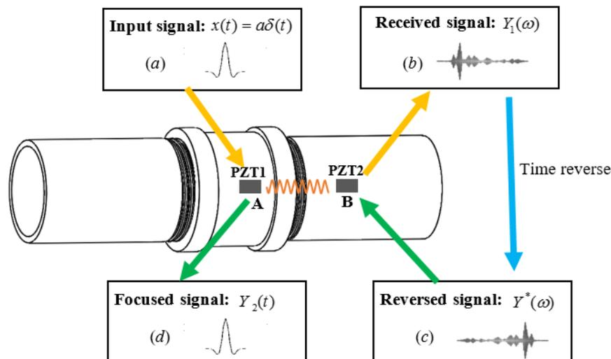
Figure 5. Theoretical procedure of time reversal technique.
