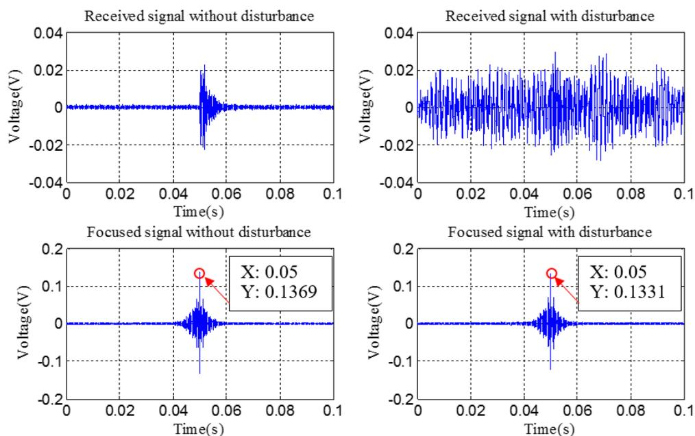
Figure 13. Anti-disturbance ability test with a loosening rotation angle of 30°.
