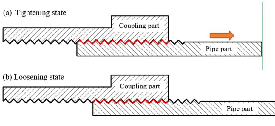
Figure 3. The reduction of the contact area for the connection interface caused by pipe looseness.
