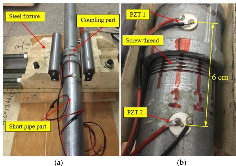
**Figure 6.** The test specimen of threaded pipe connection and the PZT sensors. (a) The test specimen; (b) The location of PZT sensors.
