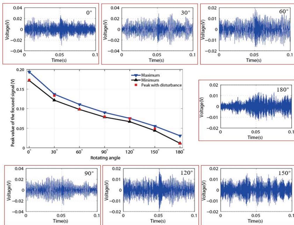
Figure 14. The anti-disturbance ability test for each loosening severities.
