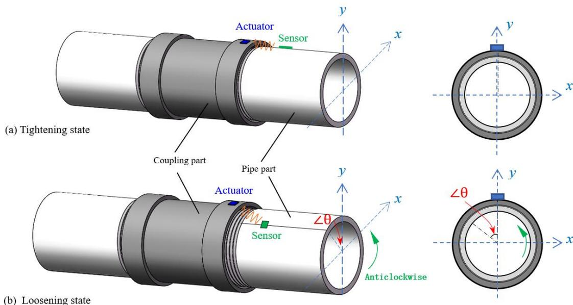
**Figure 2.** The schematic of the stress propagation between the lead zirconate titanate (PZT) actuator and PZT sensor on threaded pipe connection.
