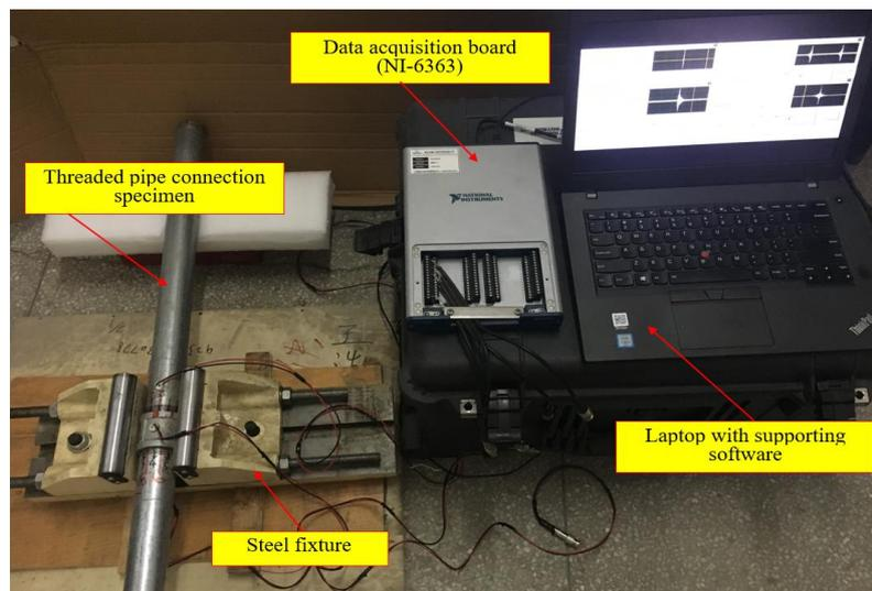
**Figure 8.** The instrumentation setup.
