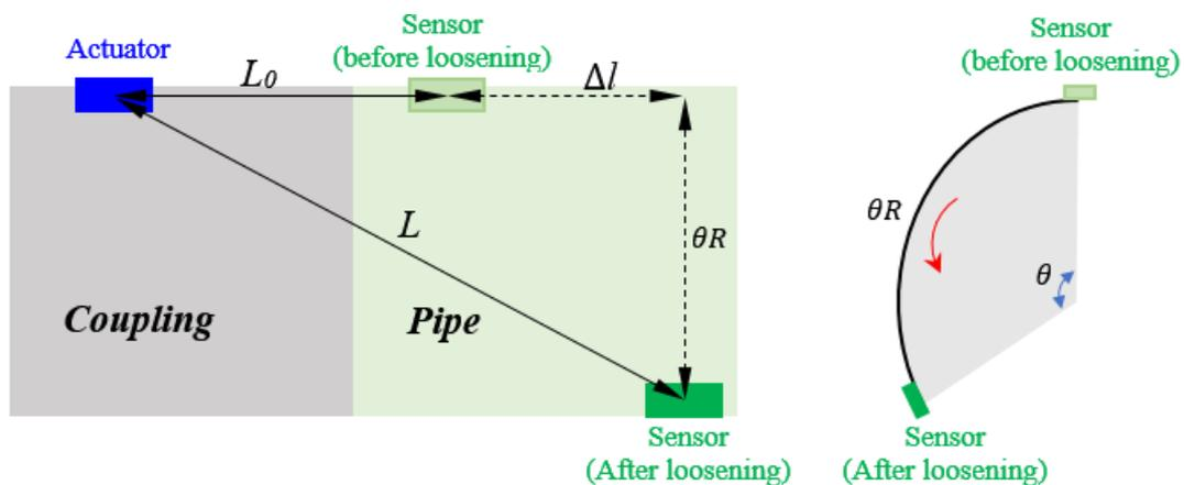
Figure 4. The change of the relative distance between the PZT actuator and sensor because of the looseness with a rotation angle  $\theta$ .
