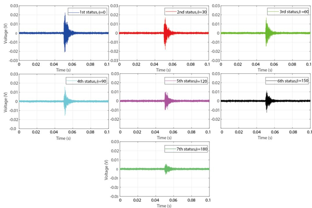
Figure 9. The wave response signal received by PZT2 in the first step.
