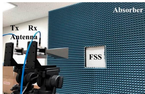
Figure 5. Frequency reflection characteristic measurement setup.
