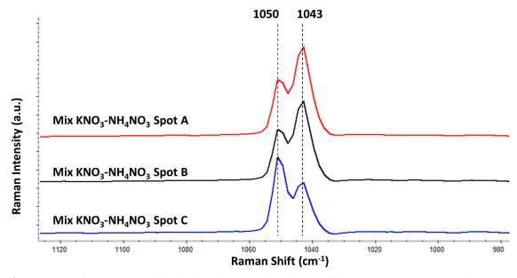
**Figure S2**. Test for experimentally checking the spectral resolution of the Raman spectrometer. The spectra were collected from different spots in a potassium and ammonium nitrate mixture. The bands of potassium nitrate (1050 cm<sup>-1</sup>) and ammonium nitrate (1043 cm<sup>-1</sup>) were resolved. All the spectra are displayed using the same scale, but they are vertically offset for clarity.
