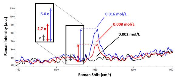
**Figure S3**. LOD estimation for nitrate, according to its most intense Raman band (1049 cm<sup>-1</sup>). As evidenced, the Raman intensity for the 0.016M solution exceeded three times the signal-to-noise ratio (5.0), whereas the Raman intensity for the 0.008M solution was almost three times the signal-to-noise ratio (2.7). No nitrate band was perceptible for the 0.002 M concentration. All spectra are displayed using the same scale and no vertical offset.
