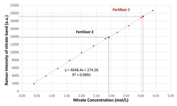
**Figure S4.** Quantification of the nitrate concentration in the fertilizers by interpolating the Raman intensity of the nitrate band of those fertilizers (Figure 4). The interpolation was performed on the calibration line prepared from different nitrate solutions (4.4 to 0.4 mol/L). The standard deviation vertical bars are included for each calibration measurement; however, they are not perceptible at this scale since the RSD was below 0.4 % for all the replicate measurements.
