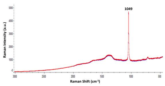
**Figure S1**. Five-replicate Raman spectra for the 1M nitrate solution collected either in static (red) or in during-flow (blue) modes. All spectra are displayed using the same scale and no vertical offset.
