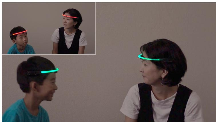
**Figure 1.** *FaceLooks*: wearable devices measuring and visually representing face-to-face behavior in real time.
