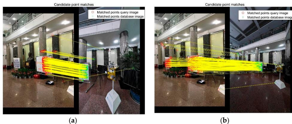
**Figure 6.** Matches after geometry check. (a) Most matched image with 390 matches. (b) A uniform distribution with 339 matches.
