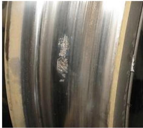
Figure 11. An example of the bogie fault (wheel tread peeling).
