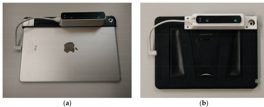
Figure 2. Hardware used in the SIRAE project consisting of an iPad and a Structure Sensor (a); and the devices protected with cases (b).
