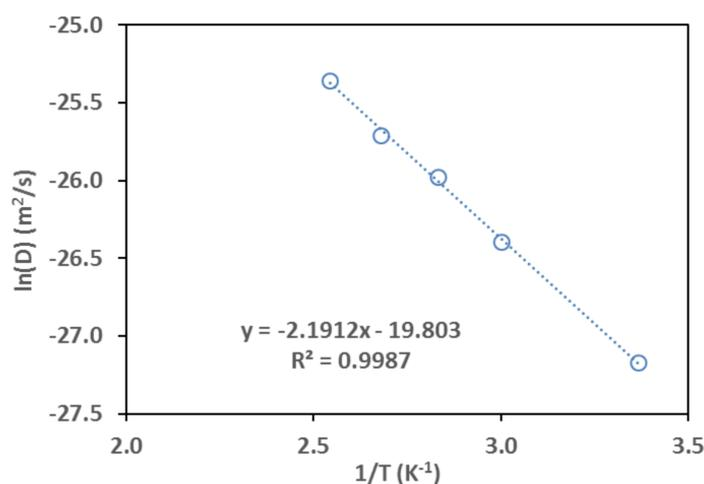
Figure 14. Arrhenius plot of isobutane diffusivity ( $D$ ) obtained by the FOI sensor.
