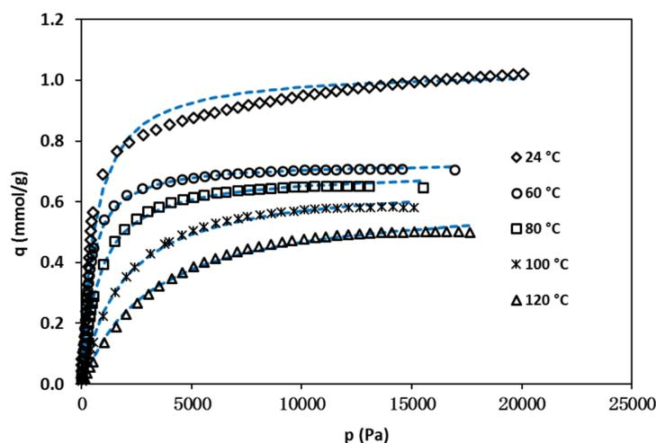
**Figure 6.** Isotherms of isobutane in silicalite at various temperatures (dashed lines are least square regressions using the extended Langmuir equation).
