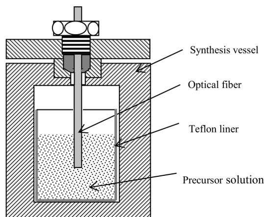
**Figure 2.** Schematic showing the cleaved fiber end mounted in the synthesis vessel.
