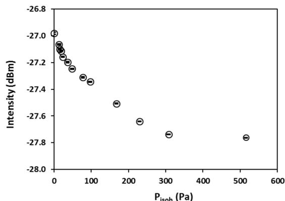
**Figure 8.** Correlation of the zeolite film-coated FOI reflection intensity at a fixed wavelength of 1566 nm with the  $P_{isob}$  at 24 °C.
