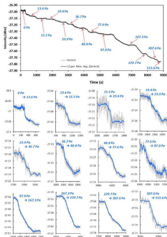
**Figure 9.** Temporal response of single wavelength ( $\lambda = 1566$  nm) intensity to staircase variations of  $P_{isob}$  (the top figure shows continuously monitored response and the small figures underneath are temporal response to each of the staircase changes).
