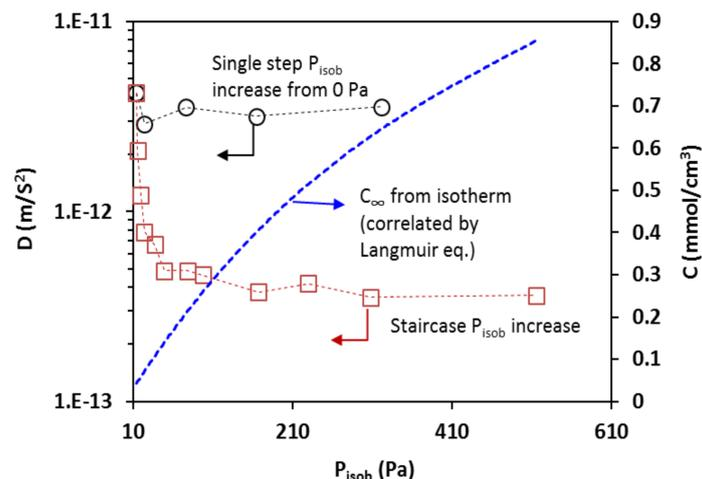
**Figure 11.** The transport diffusivity measured under the two conditions shown as a function of  $P_{isob}$  together with the corresponding isobutane equilibrium concentration in the zeolite.
