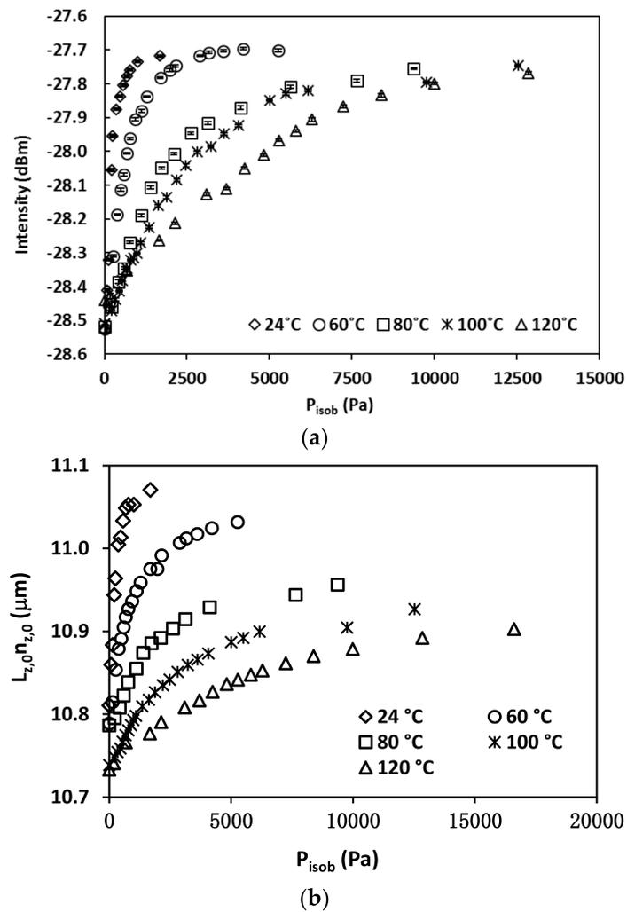
**Figure 13.** The pressure ( $P_{isob}$ ) dependence of (a) reflection intensity at a fixed wavelength of 1574 nm, and (b) zeolite film optical thickness ( $L_{z,0}n_{z,0}$ ) at various temperatures.
