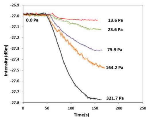
**Figure 10.** Temporal responses of reflection intensity at  $\lambda = 1566$  nm to one-step  $P_{isob}$  increase from 0 Pa to various specific values.
