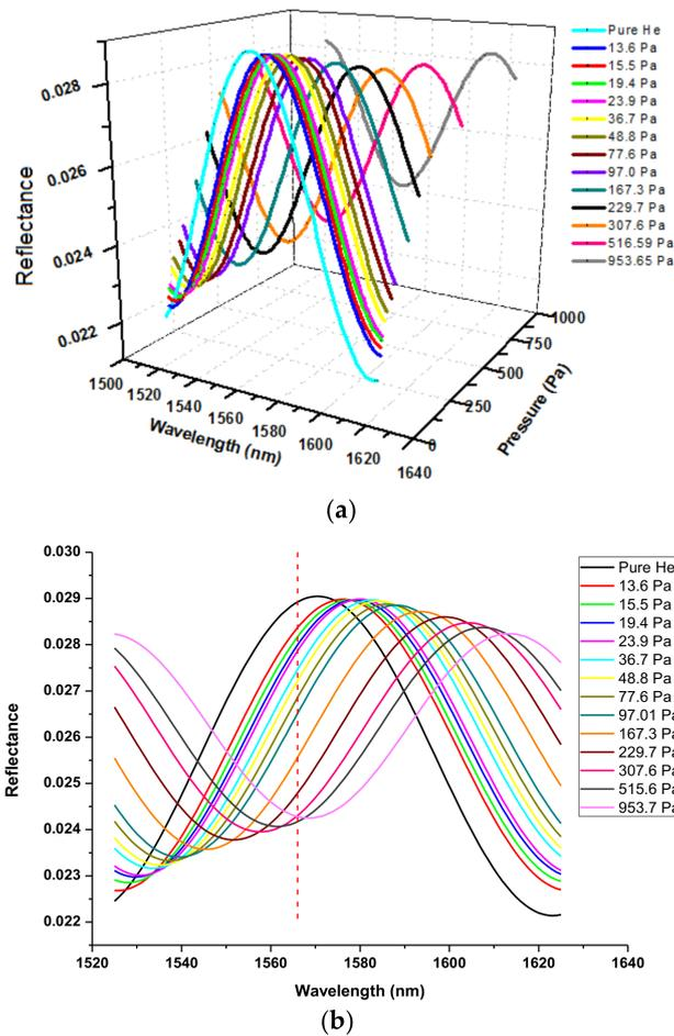
**Figure 7.** Interferograms of the zeolite film-coated FOI sensor under equilibrium states at various  $P_{isob}$ : (a) 3-D presentation and (b) 2-D view of interference evolution with equilibrium  $P_{isob}$ .
