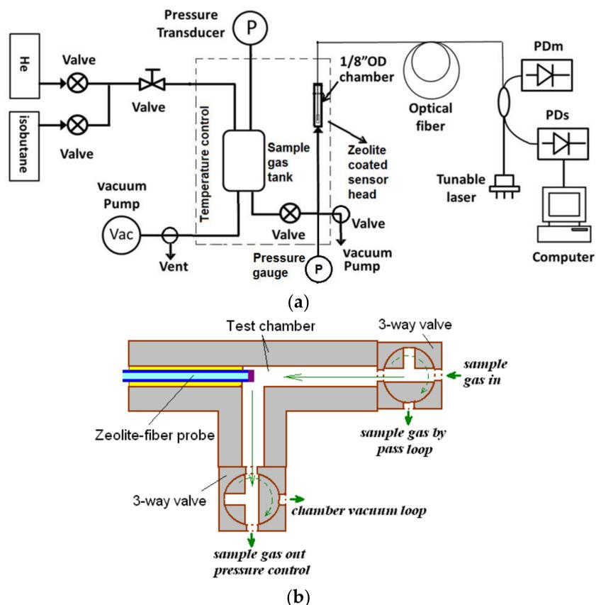
**Figure 3.** Schematics showing (a) the experimental system for FOI sensor operation; and (b) the FOI sensor head installation in the testing chamber.
