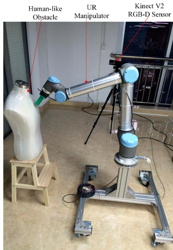
Figure 5. Experiment setup. UR represents Universal Robots.
